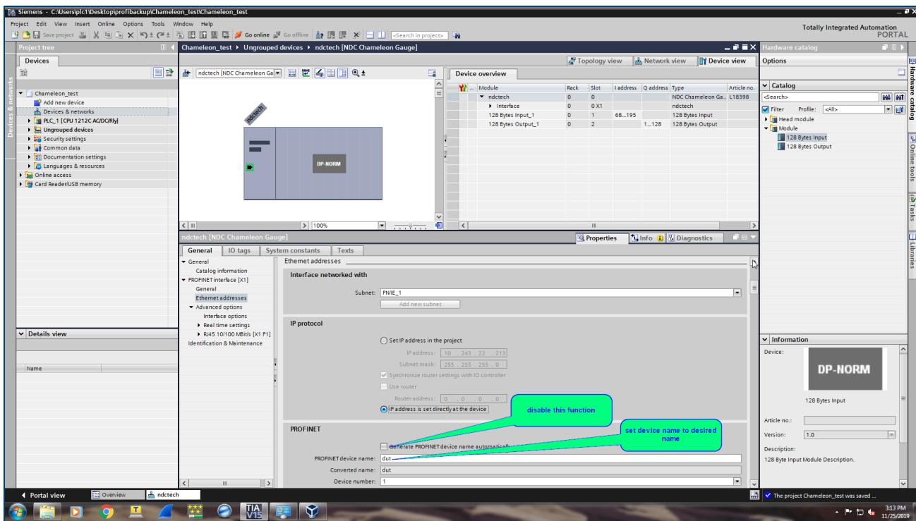
To use the Device name specified in the GSDML file, enable the **Generate PROFINET device name automatically** box. Alternatively, to use a different name, disable the automatic naming function and enter the desired name in the **PROFINET device name** line.
