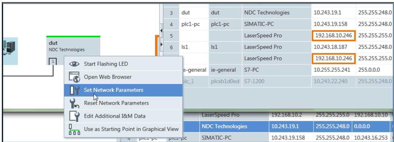
3. From the Set Network Parameters pop up window, you can change the device name and ip settings.
