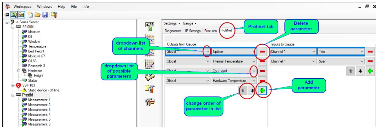
3. Add or remove parameters by clicking on the + or – buttons, or use the drop down boxes to select the parameters.
