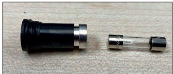
Figure 8-8 Pull out and replace fuse
