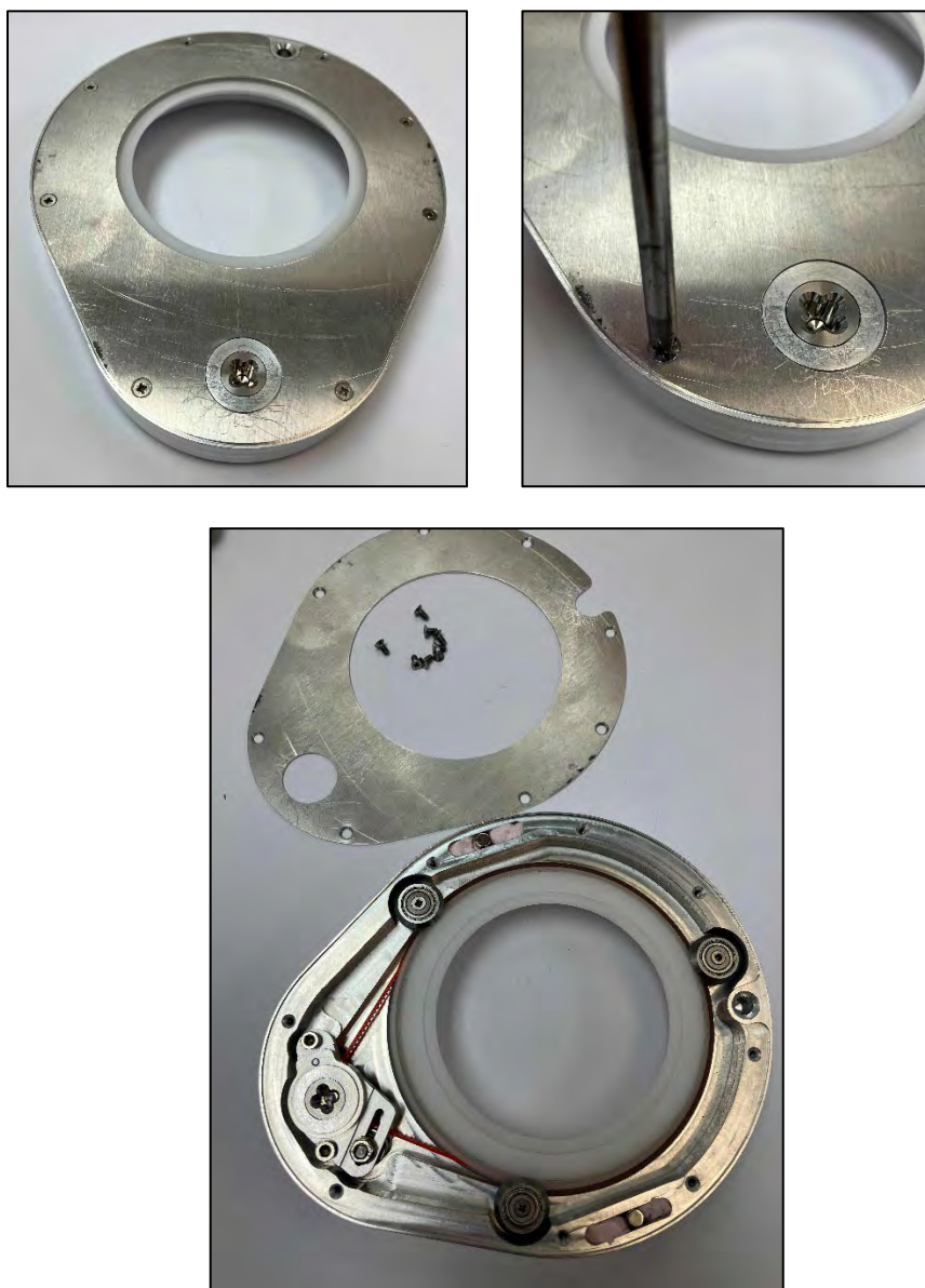
Figure 8-3 Remove the cassette rear plate
