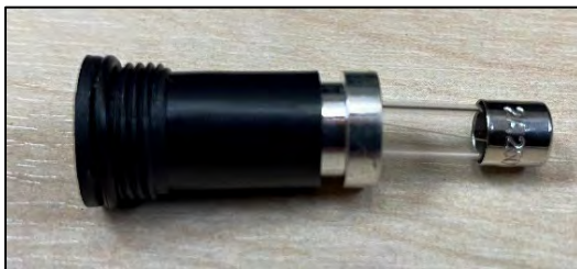
Figure 8-8 Pull out and replace fuse
