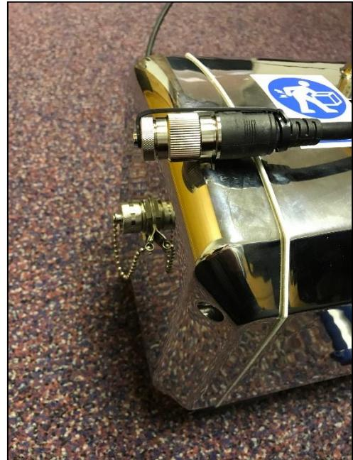
To prevent the sensor plug/socket from being easily disconnected without a tool, the connector clamp must always be fitted as shown in the photo above as follows:
