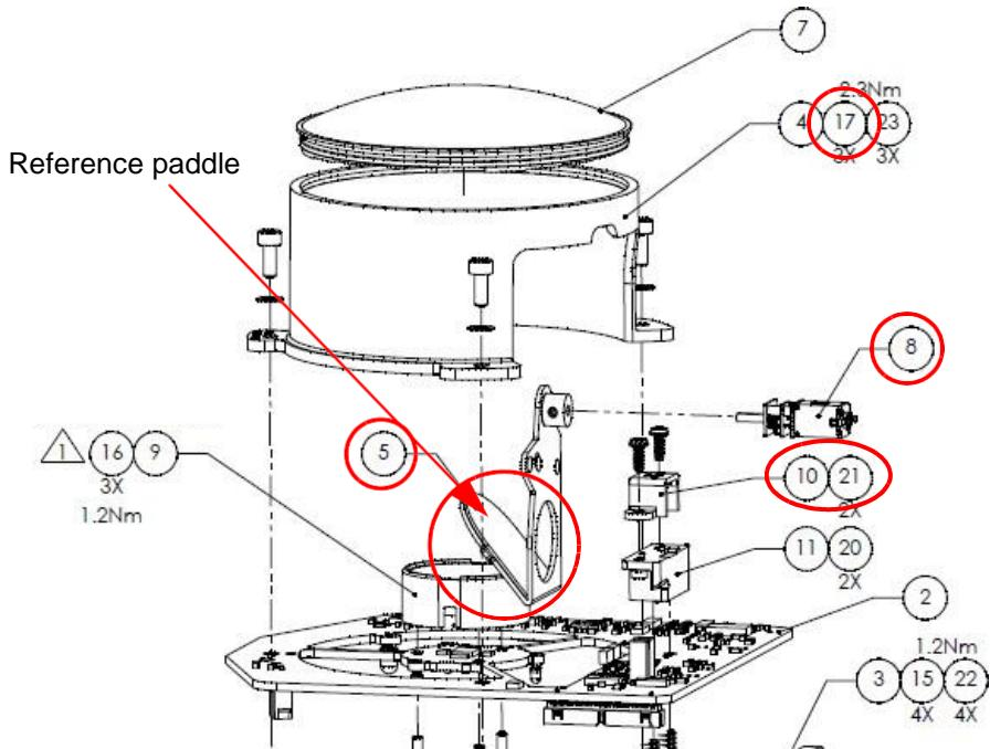
7. Carefully unplug the motor lead and remove the two pozi drive screws securing the reference motor clamp (8, 10, 21) and lift away the motor and reference paddle (5).
