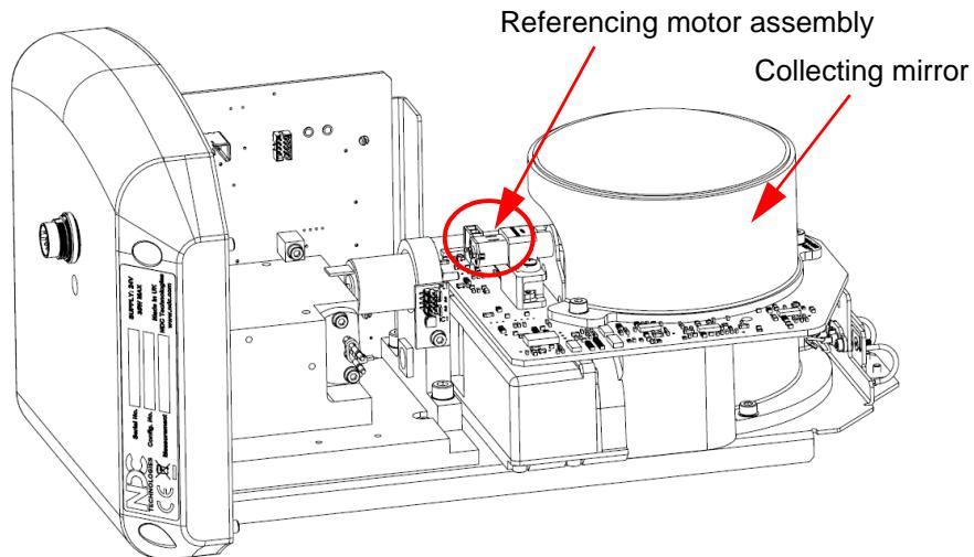
6. Remove the collecting mirror by removing the 3 x M4 screws (item 17 below) with a 3 mm Allen key, then carefully lift and store it away.
