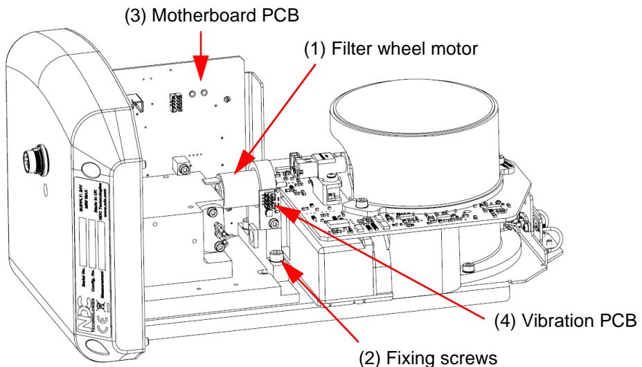
6. Unplug the filter wheel motor ribbon cable connector from the motherboard PCB (3).
