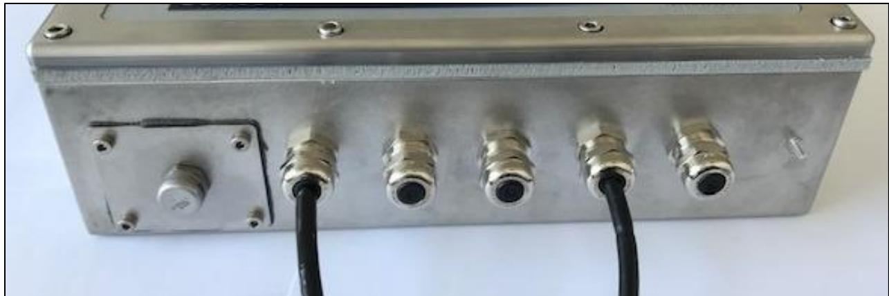
ATEX certified glands are fitted with integral ATEX certified blank inserts that should be kept in place to ensure the seal. In order to ensure that the enclosure is sealed, these inserts should only be removed when replaced with cables.
