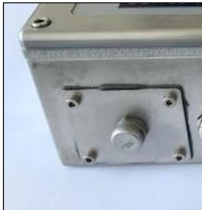
To expose and use the RJ45 port, remove the metal cover by unscrewing the four M4 retaining screws with a 3.0mm Allen Key. **Note that this can only be done when the explosive atmosphere is NOT present.** Always refit the cover and tighten the 4 x screws to a torque of 1.0Nm using a 3.0mm Allen Key torque wrench.
