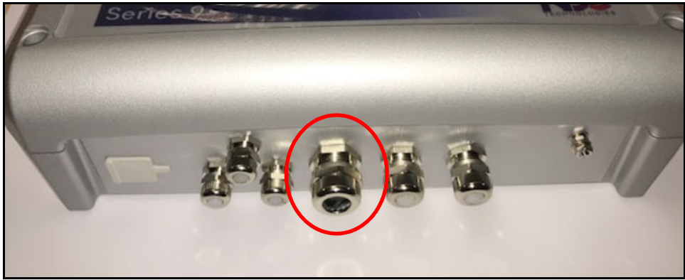
Figure 9-29 Connect cable to large cable gland on Series 9 peripheral
