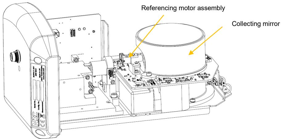
Remove the collecting mirror by removing the 3 x M4 screws (item 17 below) with a 3mm Allen key and carefully lift away and store carefully.
