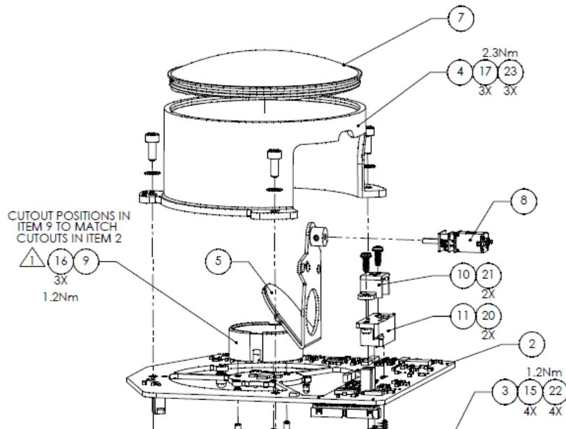
Carefully unplug the motor lead and remove the two pozi drive screws securing the reference motor clamp (8,10,21) and lift away the motor and reference paddle (5).
