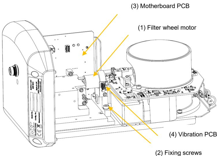
Unplug the filter wheel motor ribbon cable connector from the motherboard PCB (3).
