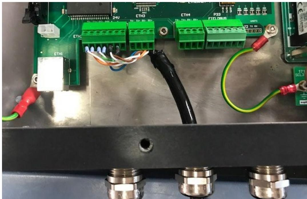
To clamp the cable securely and form a good seal, the gland nut must be tightened with a 20mm A/F torque wrench to 3.5Nm.
