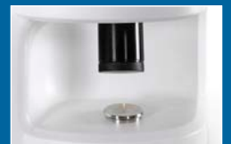
Reference standard for routine stability checks and standardization after servicing
